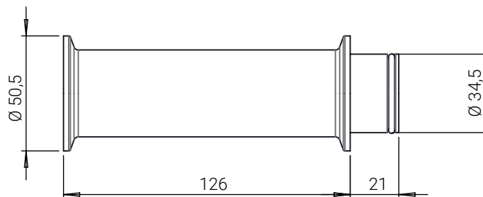
The overall diameter of the UKK is 50,5 mm. The distance between the tri-clamp connections is 126 mm.
